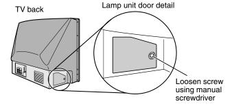
Using a manual Phillips screwdriver, loosen the two screws on the lamp unit.
